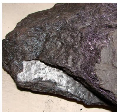
Figure 2 – Fluid solidified on the interlayer surface (bed m_3 , O.F. Zasyadko mine)
